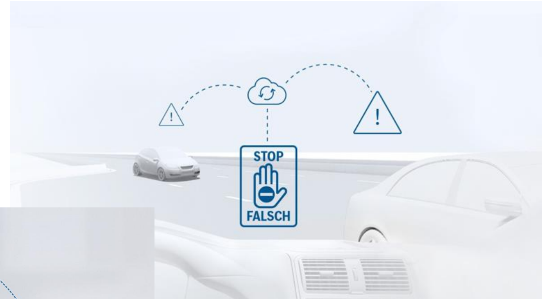
Cloud-based wrong-way driver warning
